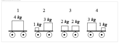
Each of the four identical carts shown above is loaded with a total mass of <sup>4</sup> kilograms. All of the carts are initially at rest on the same level surface. Forces of the same magnitude directed to the right act on each of the carts for the same length of time. If friction and air resistance are negligible, which cart will have the greatest velocity when the forces cease to act?
